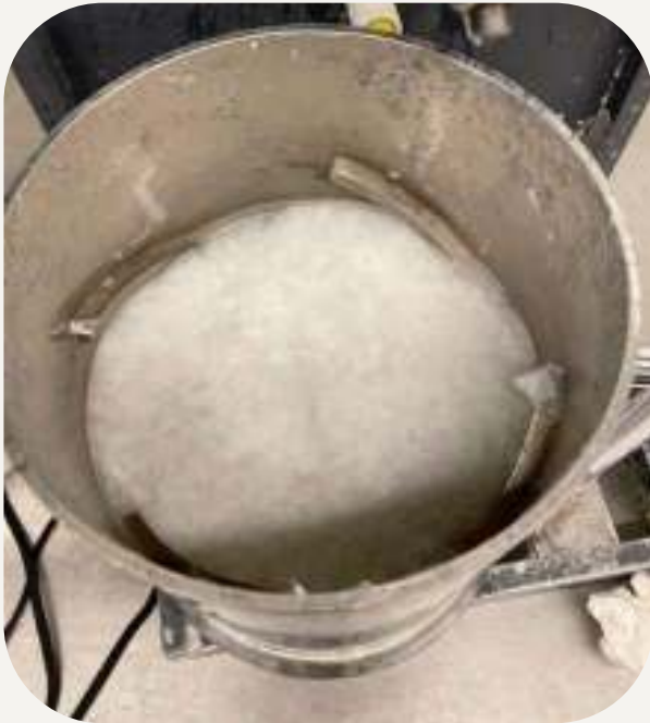
Above: Sample deflaked on disintegrator.
