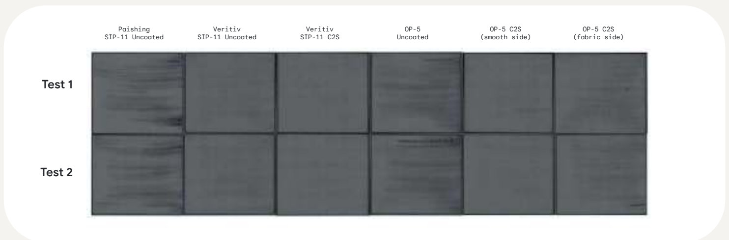
Above: Abrasion on a common enclosure material using a Sutherland Rub tester.
