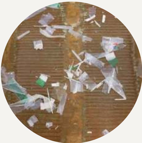
Above: Plastic film removed / separated in a mill's hydropuller (repulping) system.
